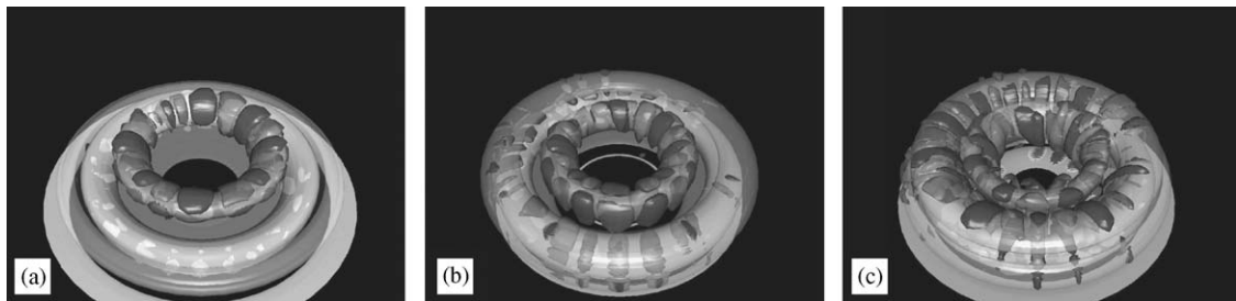
Fig. 10. Development of the azimuthal instability after a vortex ring impact with a wall at Re_\Gamma = 2895 . (a) t^* = 30 , (b) t^* = 37.5 , (c) t^* = 45 .
